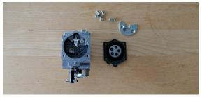
remove the semi-circular plate, opening the 2 screws
