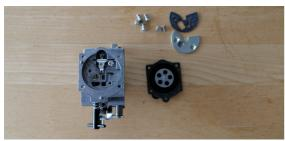
remove the paper gasket also. Use a small sharp screw driver to get it out as it may stick, but use precaution not to damage it!
