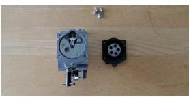
open cover by removing the 4 screws, put cover and gasket incl. lever plate aside. You need to slide out the nipple from the fork of the lever to be able to remove the plate. Use precaution here not to bend the lever or damage / misshape the lever plate!
