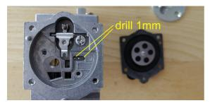
you can find 3 small holes in the shown oval window. The middle one should remain unchanged, the 2 other ones each enlarge by drilling with a 1mm (metric) drill (use regular metallic drill with portable drilling machine)
